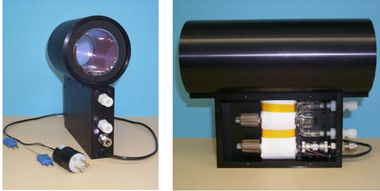
Figure 3. Typical iodine filter (cell) configuration [Ref. 30].
